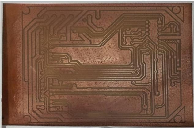
Fig 9 Example of the etched PCB after paint stripping process.
