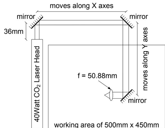
Fig. 4 Setup of CO<sub>2</sub> laser based system.
