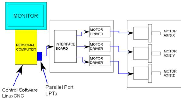
Fig. 3 Block diagram of the CNC system.
