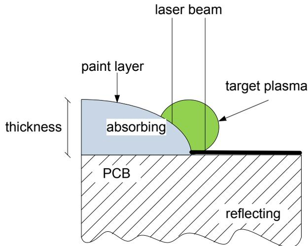
Fig. 8 Laser stripping process.
