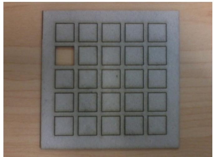
Fig. 7 Reproducibility and accuracy of 10x10mm<sup>2</sup> squares using laser cut. We got WYSIWYG result.
