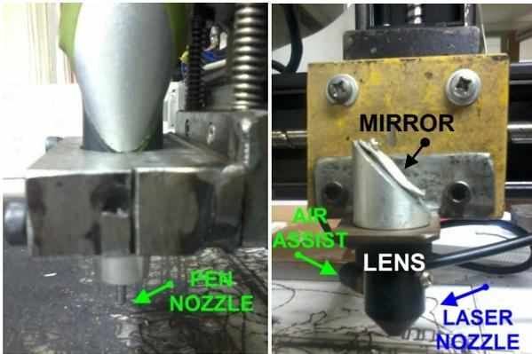
Fig. 5 The head was mounted along the Z axis. From left to right: impact-engraver-pen and mirror-lens.
