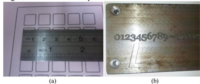
Fig. 1 Engraving result on (a) paperboard target using inked-pen with rectangle 10x10mm<sup>2</sup> and (b) metal target, i.e. iron, using impact-engraver-pen.
