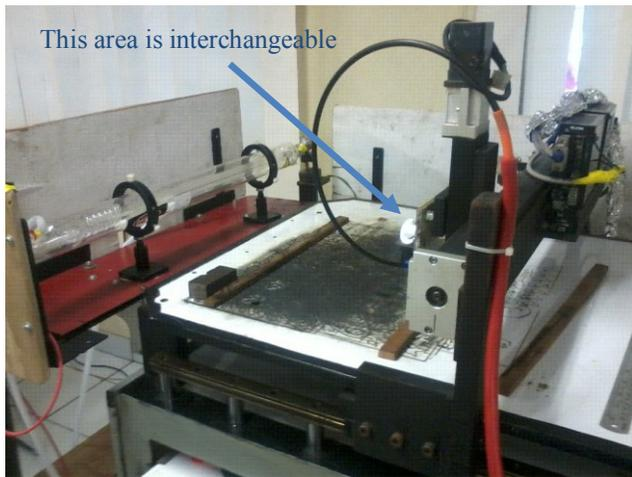
Fig. 2 Manually interchangeable cutting head of homemade CNC.
