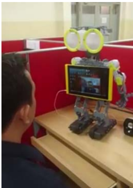
Fig. 1. Intelligent humanoid robot for teaching Mathematics in Indonesian language. The face and speech recognition systems developed using Python and OpenCV [17]
