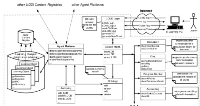
Figure 6. Components of a distributed, Web-Services-Based LCMS
