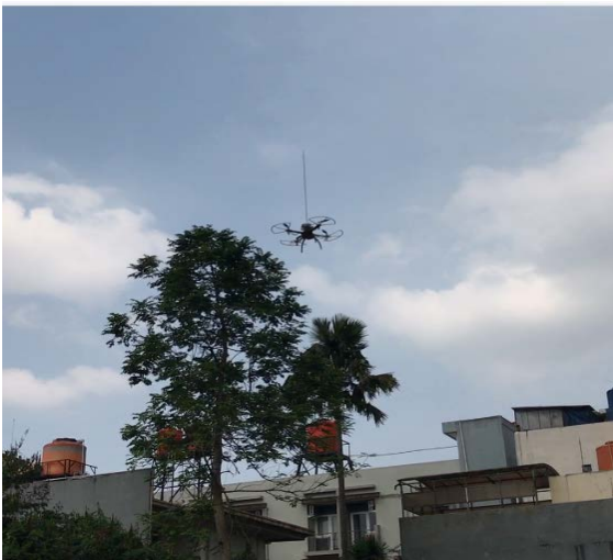
Fig. 14. Quadrotor slows down to move left as the error of roll angle of inverted pendulum becomes smaller
