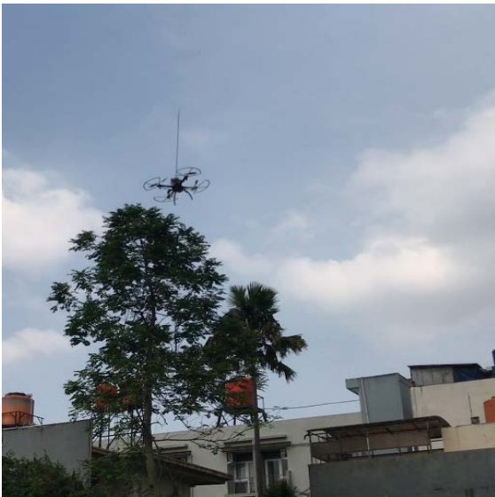
Fig. 13. Quadrotor then moves left to stabilize the inverted pendulum
