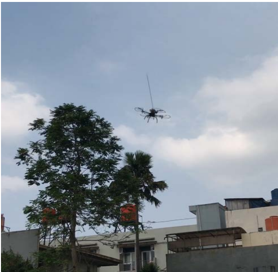
Fig. 12. Quadrotor still moves to the right while inverted pendulum roll to the counterclockwise
