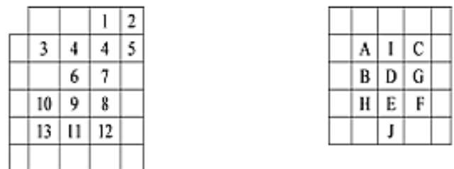
Fig. 6. Facility and Machine Corelap Allocation Pattern
